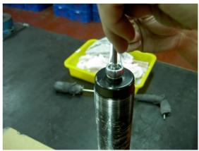
4) Pull out the inner cylinder gently. The bump stopper will appear. Separate the inner cylinder from the outer cylinder.
