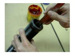
14) NOTE Please ensure the new lubricating oil or grease is well covering the inside surface of cylinder in order for maximum performance of shock. The new oil should cover entirely over all 4 Oilless Bearings inside the tube. And need to be about 30mm extend below the bottom oilless bearings. And apply large chunk of lubricating oil at the oil seal opening.
