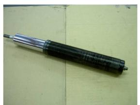
2) Please see the bottom of the cylinder. There should be a tightened hex nut.
