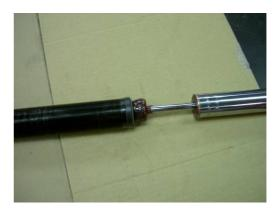
5) Remove the bump stopper from the inner piston rod.
