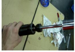
16) Insert the inner cylinder until the striated tip is through the outer cylinder. Then screw the hex nuts and washer back to original place.
