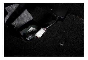
Plug the Male connector housing now back into the 4WD and secure the Syvecs 4WD module on top of the OEM ECU with double sided tape.
